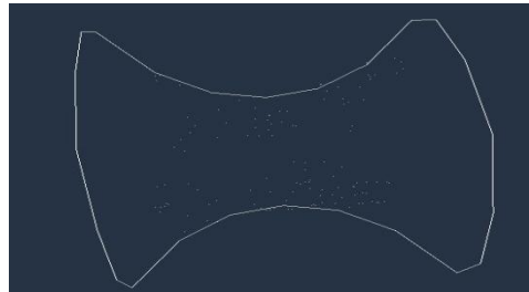
Fig. 7(3) Error analysis from different perspectives, large or small errors denoted by dense or sparse sets of points
